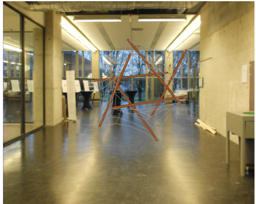
Figure 6: Impression of the tensegrity model rolled over
