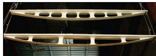
Fig. 6. Producing Beam with fabric formwork [3]
