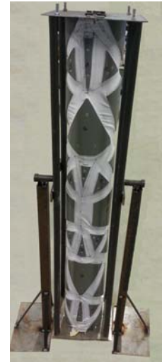
Fig. 15. Mould and falsework for the concrete scale models
