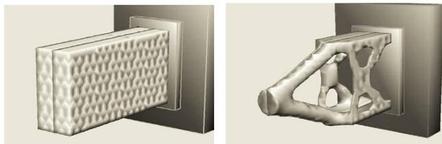
Fig. 4. Optimization of cantilever with ESO <sup>26</sup>.
