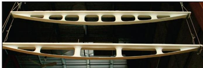
Fig. 6. Optimized beam with fabric formwork <sup>3</sup>
