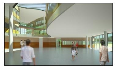
The positive point of the flexibility is the application of lightweight partition walls and the column free aula in the centre of the building. The makes it possible to change the form of the rooms, as far as possible because of the column structure.
